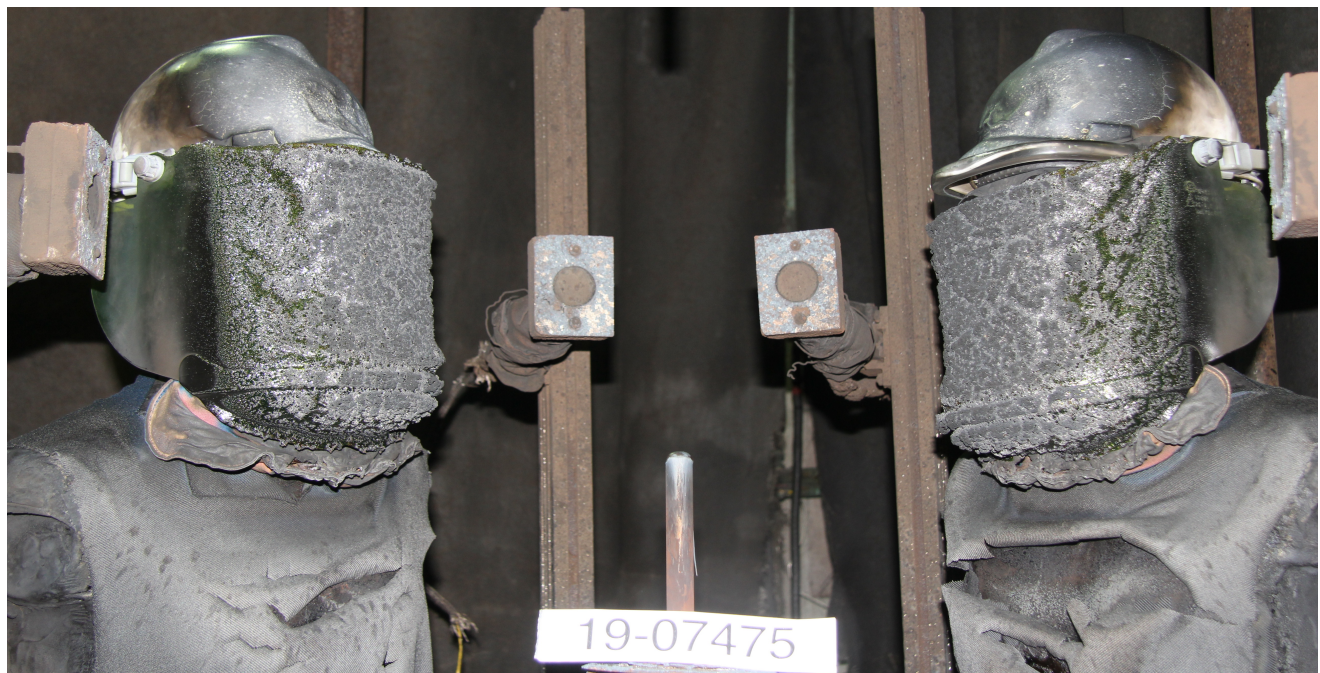
Figure 2. Hood system after arc exposure at 92 cal/cm 2
